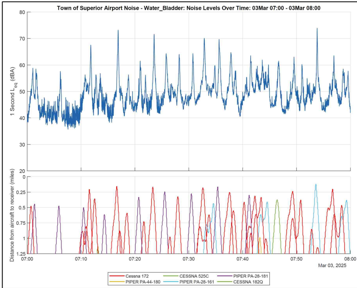
Figure 3 – Noise Levels and Aircraft Operations during an Example Hour on Median Day (Water Bladder)
