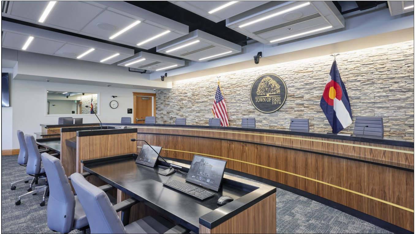
Council Chambers dais, where bullet-resistant protection is provided. The chamber has a second entrance and a dedicated emergency exit.
